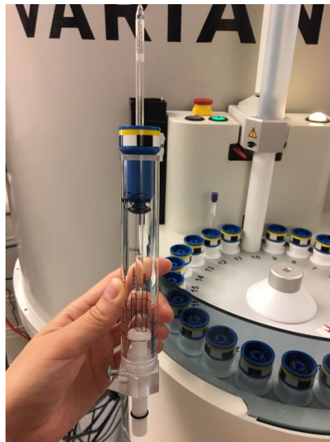
Figure 3. Placing the sample into the spinner using the depth gauge.
